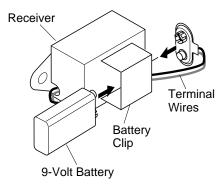
Figure 46 - Installing Battery in Receiver
